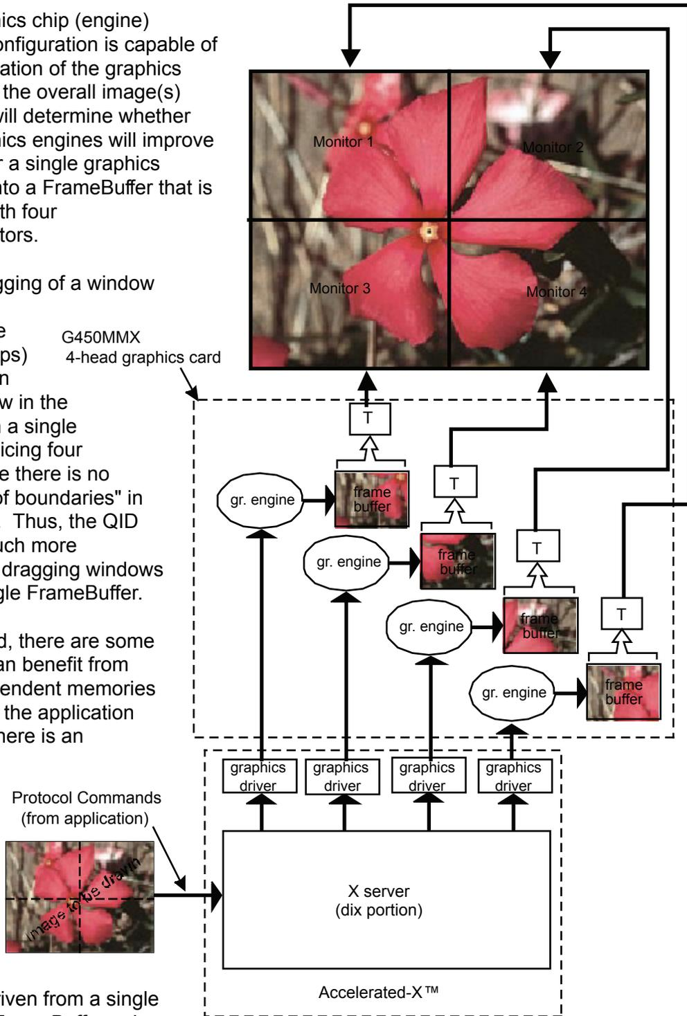
Drawing (and other) commands are sent to the X Window System X server (the device independent part of the X Window System) via "X Protocol Packets" by an application. Those packets are interpreted by the X server and executed to generate the display. Obviously, the graphics system configuration is very important here.
