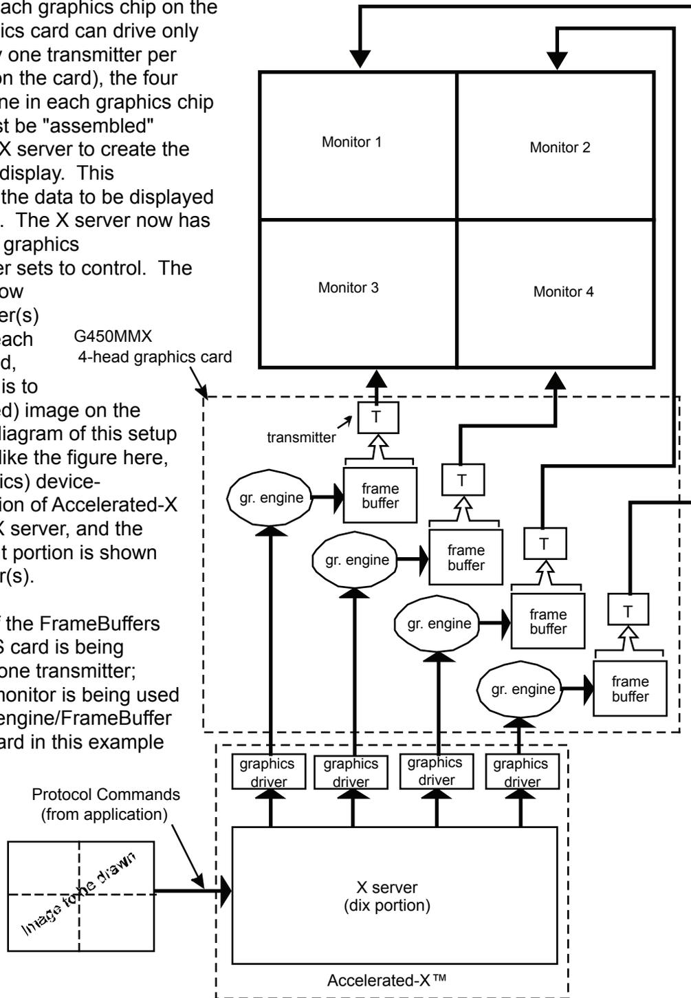
Here is the previous block diagram with some "color" added. (Clearly, no one would generate such an image using X11 Protocol drawing commands - but the jpeg images are pretty and show the desired effect).
